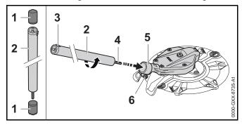
► Remove protective caps (1) from both ends of the drive tube (2).
