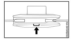
If one of the wear limit marks on the PolyCut mowing head is worn through (arrow): Do not continue using the mowing head. Install a new one. There is otherwise a **risk of injury** from thrown parts of the head.
