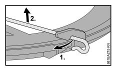
Disconnect wire rod from the transport guard.
